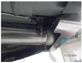
**Step 5.** To retain the OEM tips on your vehicle select the two OEM Tip Assemblies. The drivers side will be slightly longer. Loosely attach each pipe inlet to the Over Axle Pipes outlets using the OEM clamps. Engage the welded hangers for each to the rubber insulators.
