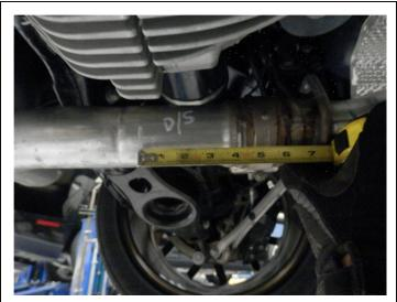
**Step 1.** Begin removal of the OEM system by cutting both side of the systems exhaust pipes. For the drivers side cut 4" rearward of outlet weld on the exhaust control valve as shown in the attached picture.
