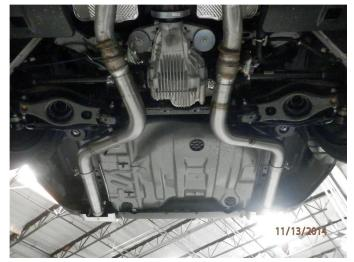
**Step 4.** Begin installation of your new system by slipping each Inlet Pipe Assembly over the cut OEM outlet pipes. The drivers side pipe can be identified as the shorter of the two pipes Loosely secure using the supplied 2.75" clamps. At this point you have two options for tips. Magnaflow supplies a Quad tip setup or an extension pipe assembly to allow the original OEM tips. Select the desired option before continuing the installation.
