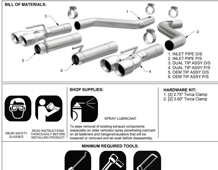
Hanger Tool (Or Pry Bar) 15mm 13mm
