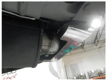
**Step 3.** Next, loosen the band clamps attaching the rear muffers to the OEM tips. You may now remove the rear exhaust system. Disengage all welded hangers from the rubber insulators. Once the two mufflers are removed from the vehicle detach the OEM tip clamps by gently breaking the welds securing them Do not discard or damage the clamps or rubber insulators as they will be used to install the new exhaust system.
