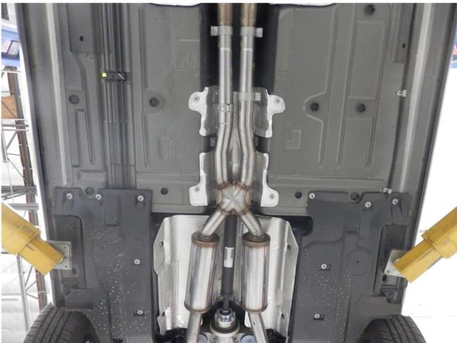
**Step 2.** Begin installing of the new system by attaching the Driver and Passenger side (Passenger is the longer of the two pipes) inlet pipes to the outlets of the OEM system using the supplied 2.25" clamps. Next attach the Resonator Assembly to the inlet pipes with supplied clamps and insert the hangers into the rubber insulators.
