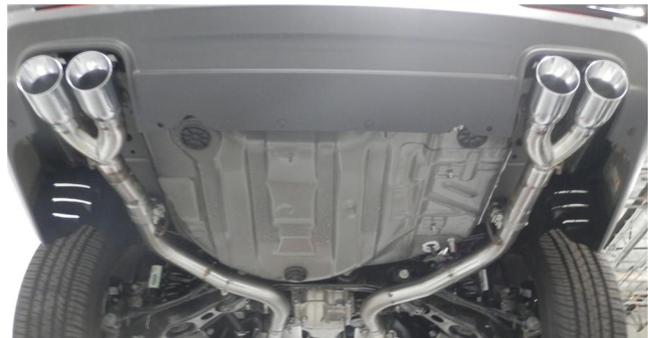
**Step 4.** We also supply a Quad tip setup that requires removing the tip surrounds located in the valance. Once removed the quad tips are routed into the openings.
