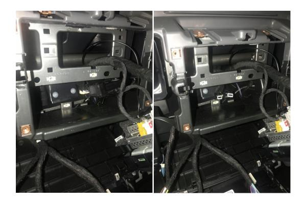
Step 8: Plug in Security Bypass Block into Existing Connectors and tuck up inside.
