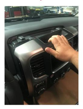
Step 4: Remove the four fasteners securing the Radio to the instrument panel
