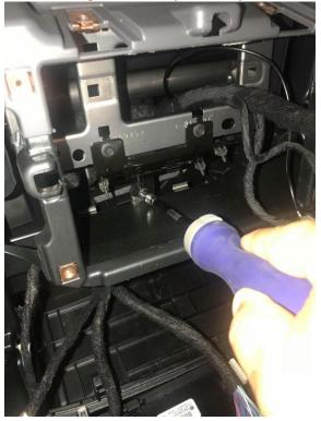
**Step 7: Unplug connectors going into Security Gateway Module (1)**
