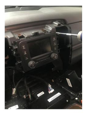
**Step 5: Remove the radio from the instrument panel.**
