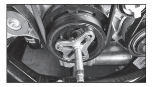
The OEM crankshaft does not have a keyway. The ATI Super Damper comes with a keyway and ATI offers a drill pin fixture kit (ATI PN918008-1) to install a pin to engage the keyway. ATI highly recommends pinning the crank. With boost, there is added resistance and the pin is necessary to prevent the damper hub from spinning on the crank snout. *There is NO warranty on cracked, spun or damaged hubs if the pin kit is not used!*
