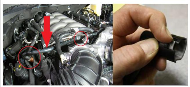
Locate 10mm bolt/stud that holds down coolant expansion tank on driver side fender. Remove bolt.
