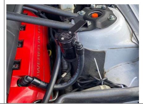
To properly clean the filter in the Oil Separator, spray any degreaser or solvent through it and let it air dry. Clean it every 10,000 miles.
