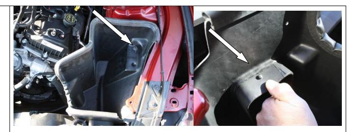
Line up duct on factory fresh air inlet and slide over. Press down on edge of duct to get the retaining "bump" past the shield.
