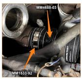
12. Slide one 105mm worm gear clamp onto coupler 3 and one on the intercooler inlet, and then install the pipe assembly from step 8 into the vehicle. Loosen the clamp from step 8 and adjust the pipe and couplers to fit properly. Ensure they have clearance around other objects, and then tighten all the clamps using a 10mm socket. Reinstall the wire from the previous step.
