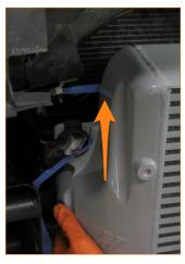
**4.** Repeat for the opposite side, then lift the intercooler to bring the bottom "C" shaped mounts up and over the lower pegs.
