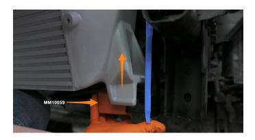
**6.** Install a bracket on each side of the lower mount and fasten using the supplied bolts (10mm socket).
