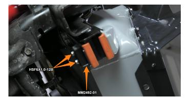
7. Install shrouds 1 and 2 using the provided bolts (10mm socket).
