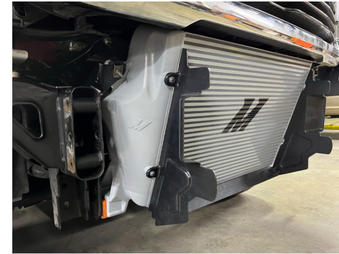
Figure 3: Mishimoto Intake Production Sample Installed
