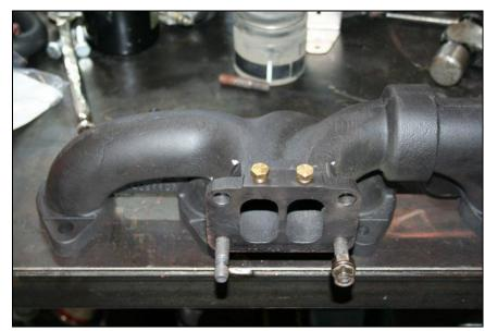
Remove factory studs from the turbo and discard. Install the provided **M10 x 1.5 x 25mm** (*1462431*) studs into the turbo.
