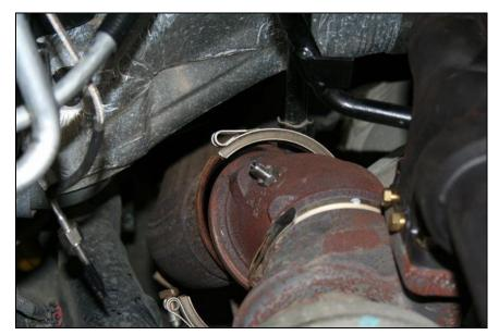
Disconnect the compressor outlet boot.
